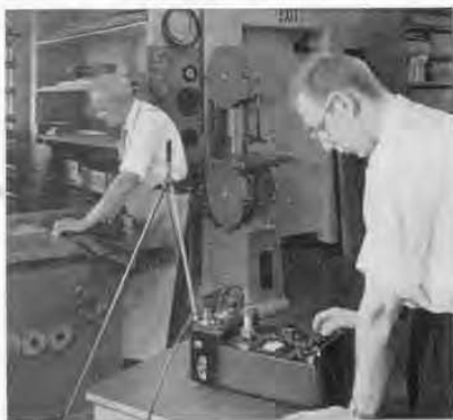
Figure 5. High-frequency sound, produced by a power saw, is measured with the sound-level meter and condenser microphone system.
